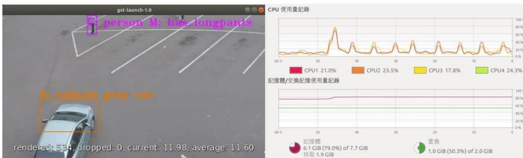
(b) DETECTION\_INTERVAL=10, RECLASSIFY\_INTERVAL=10, TRACKING\_TYPE=short-term
